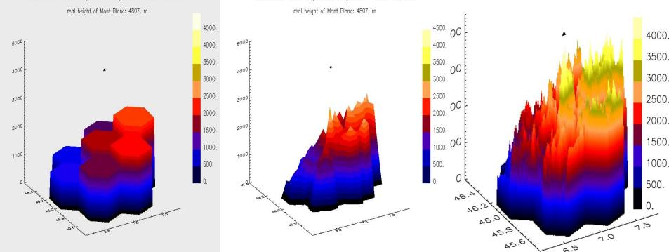
Aggregated to 40-km GME; grid element area: 1384 km<sup>2</sup> Aggregated to 7-km HRM; grid element area: 49 km<sup>2</sup> 1 km x 1 km raw data
