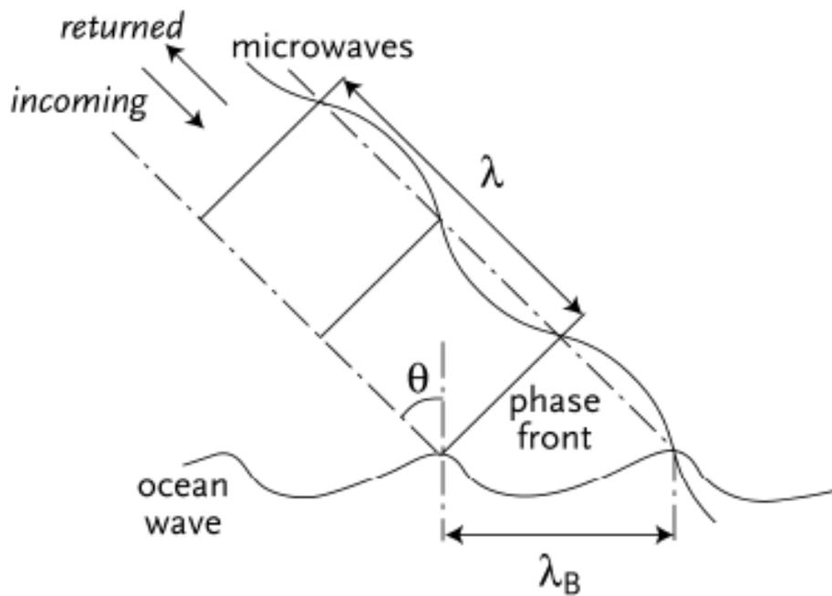
**Figure 11.** Bragg scattering: A plan-parallel radar beam with wavelength  $\lambda$  hits the rough ocean surface at incidence angle  $\theta$ , where capillary gravity waves with Bragg wavelength  $\lambda_B$  will cause microwave resonance.
